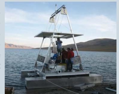
Installation of the UWITEC drill platform for taking long cores at Tangra Yumco.
